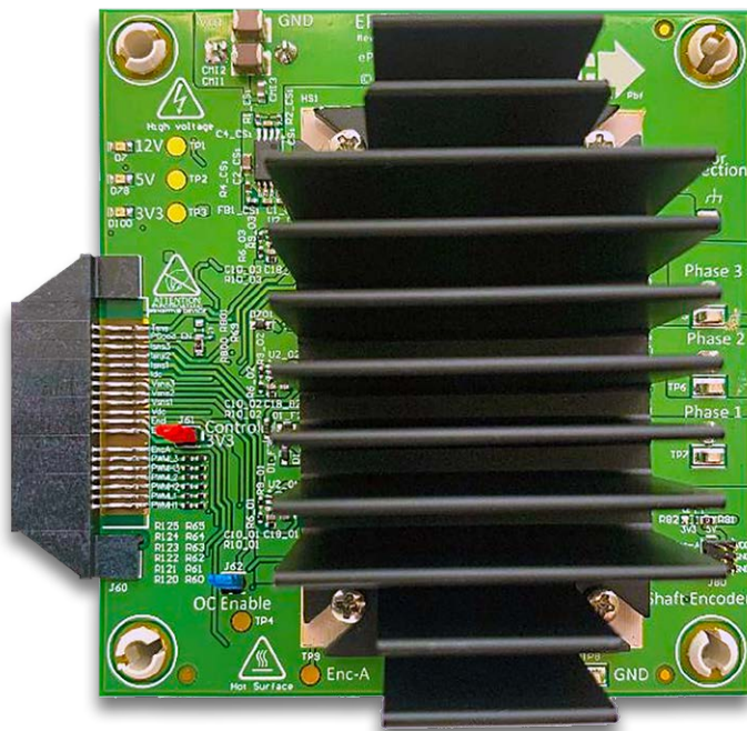
Natural Convection Cooling
